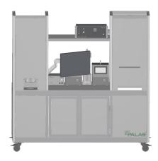
Test system for large filter elements up to a cross-sectional area of  $610 \cdot 610$  mm
