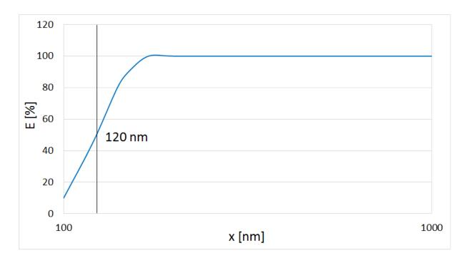
Graph 1:welas 1000 series of aerosol sensors is characterized by its very high counting efficiency starting from 0.12  $\mu$ m! Pressure-resistant and heatable aerosol sensors with a special cuvette for the variants P, H and HPmeasuring cuvettes allow the use of the welas aerosol sensors even under unusual measuring conditions. These are available:
