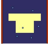
For concentrations up to 1,000,000 particles/cm³ the welas® 2070 sensor with a small measuring volume is used. This ensures the smallest measuring volume such that only one particle ever enters the measuring volume. In low concentrations, the models with a larger measuring volume offers the advantage of a higher counting rate at the same number concentration.
