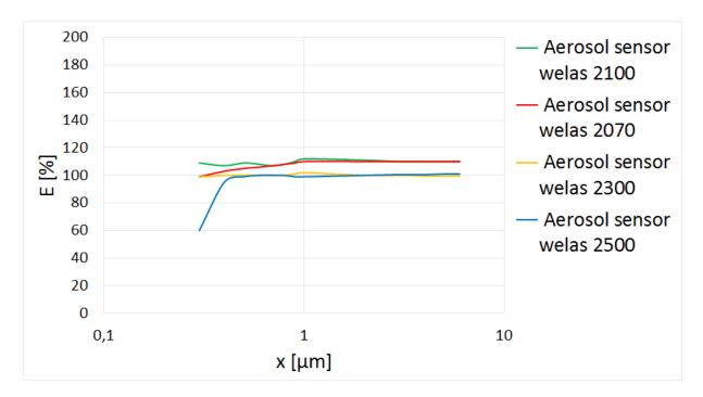
Graph 1: Counting efficiency of various sensors in relation to the welas $^{\circ}$  2200 sensor (in the measuring range 0.2 – 10  $\mu$ m) **Pressure-resistant and heatable aerosol sensors with a special cuvette for the variants P, H and HP** measuring cuvettes allow the use of the welas $^{\circ}$  aerosol sensors even under unusual measuring conditions. These are available:
