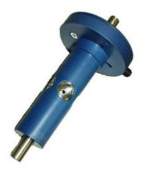
Figure 1: Heatable and pressure-resistant welas® cuvette The cuvettes are made of anodised aluminium (black). If the sensor is used in aggressive and corrosive aerosols, the cuvette can be made of stainless steel or other special materials, such as Hastelloy. Sealed additional disks prevent aerosol from the cuvette from escaping into the surroundings. The additional disks are easy to clean and replace by the operator.
