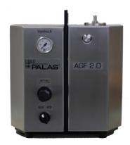
Liquid nebulizer with binary nozzle and cyclone (dp max =  $2 \mu m$ ) as per VDI 3491-1 and -2
