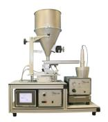
Powder disperser with weighing unit for low mass flows of approx. 8 g/h - 550 g/h; mass flow monitoring and control with automatic refill unit
