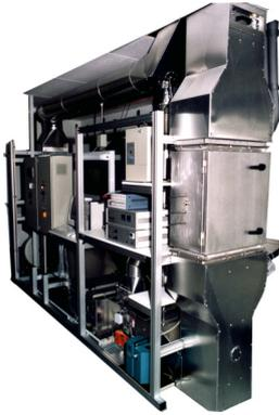
CIF 2000 test rig for standard tests on motor vehicle passenger compartment filters in accordance with DIN 71460 part 1 and ISO/TS 11155-1
