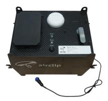
Lightweight, caseless fine dust aerosol spectrometer for integration in carrier systems, battery powered (Photo: Cased for flight drone)
