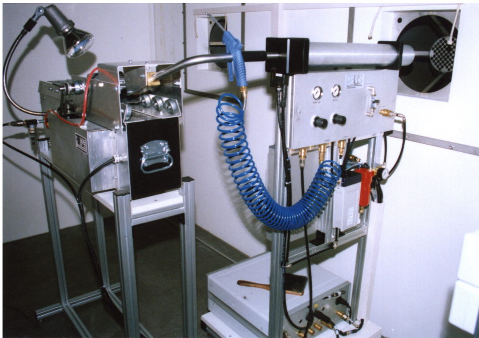
Fig. 1: Aerosol generation EN 779 Thanks to the high-resolution light scattering spectrometer Promo® 3000, the fraction separation efficiencies can be determined with greater ease, speed, reliability and accuracy. With the aid of patented optical fibre
