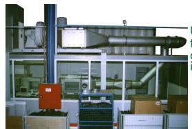
Upgrade of existing filter test channels for room air filters with aerosol technological components in accordance with EN779, ASHRAE 52.2 and ISO 16890 incl. automation
