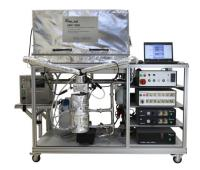
Heatable modular test system for oil mist separators better as ISO 17536
