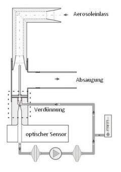
Figure 1: The schematic structure of Inas<sup>®</sup> 100
