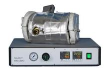
KHG 10 D dilution system heatable and pressure-resistant up to 10 bar for isothermal and isobaric dilution with a dilution factor of 1:10.
