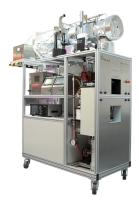
Active control of the relative humidity from 10 to 80 % and temperature from -10 to 50 °C
