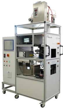
Version for testing filter media better than ISO 5011 / ISO TS 19713 engine air filters
