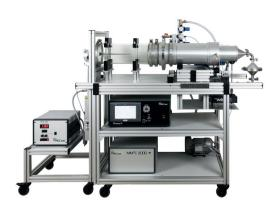
Filter test rig for cleanable filter media in accordance with VDI 3926. Versions for temperatur and/ or rel. humidity control
