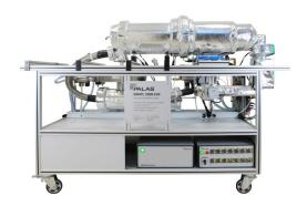
Stainless steel version with heating for temperatures up to 250°C and humidity control
