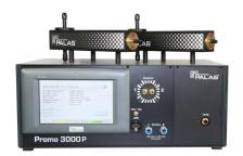
With automatic regulation of sampling volume flow by the aerosol sensors welas<sup>®</sup> under overpressure up to 10 bar
