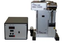
Separate dispersing unit and control unit, pressure-resistant at positive pressure values of up to 3 bar, optional low pressure operation from 300 mbar (absolute pressure)
