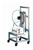
Pressure-resistant at positive pressure values of up to 3 bar, also nitrogen as a dispersing gas
