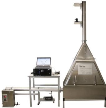
TVE 3000 for vacuum cleaner tests with dust in accordance with the standard EN 60312
