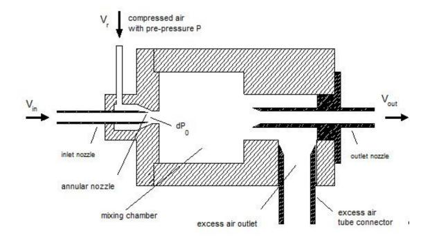
Particle-free air with the volume flow  $V_R$  circulates through an annular passage around the suction nozzle. Thus, according to Bernoulli, a volume flow  $V_{An}$  is generated at the suction nozzle. The dilution factor  $V_F$  is calculated according to the following formula
