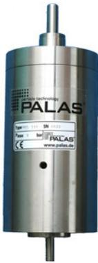
Pressure-resistant dilution system made of stainless steel for dilution at up to 10 bar counter-pressure, and for chemically aggressive aerosols with a dilution factor of 1:10.
