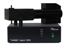
With automatic regulation of sampling volume flow by the aerosol sensors welas<sup>®</sup> under overpressure up to 10 bar
