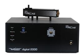
Aerosol spectrometer with an aerosol sensor, highest particle size resolution, measuring range from 200 nm to 100 µm with light wave conductor technology
